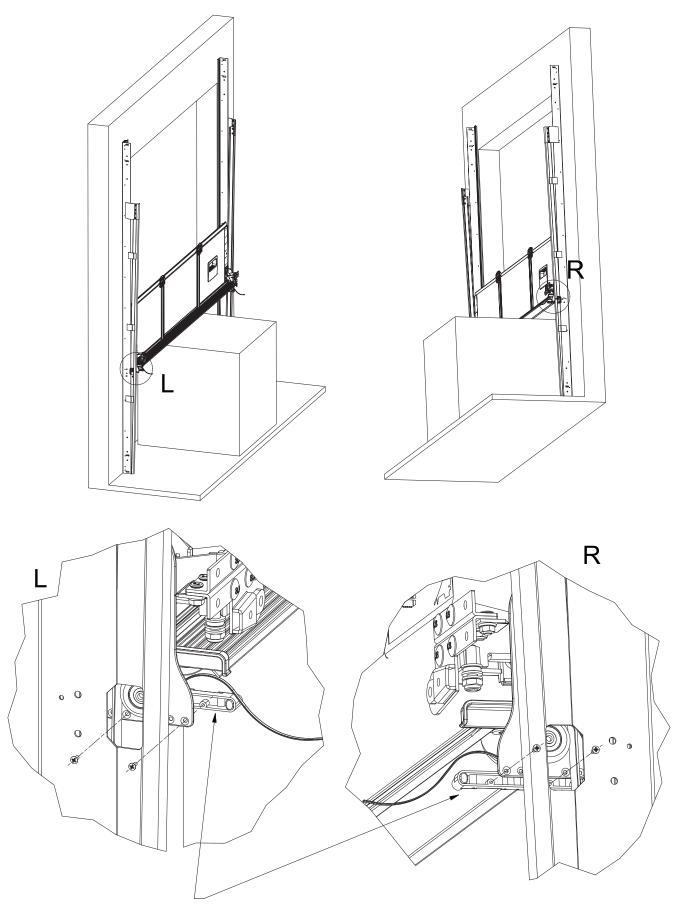
Photocell-bars (blue) are part of the safety set, packed in the operator box.
